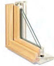
Variable thickness glass provides enhanced STC and OITC sound abatement performance. Available in Low E1, Low E2 or Low E3, tempered and obscure.
